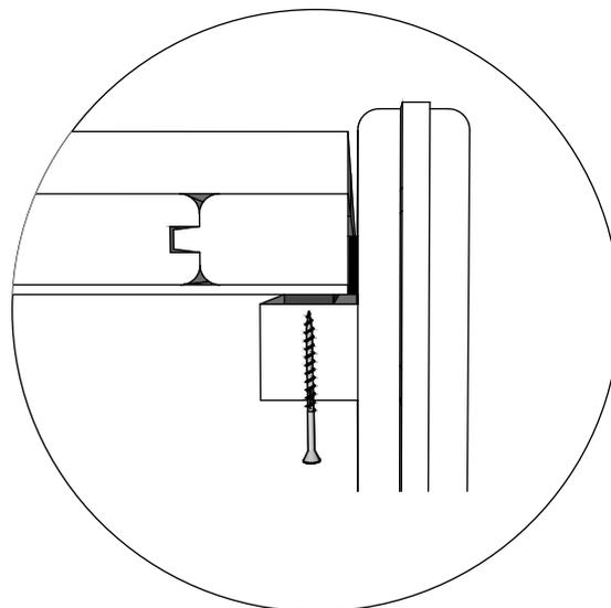
Drive the screws into the pre-drilled
