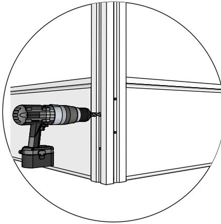
Drive the screw in pre-drilled holes
