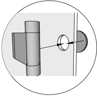
Insert the hinges into the door glass
