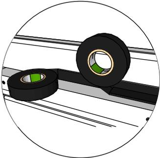
Apply sealing tape on roof panel holders
