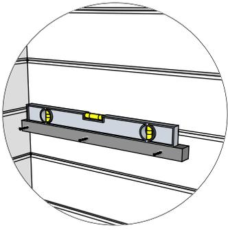
Make sure to level when installing bed holders
