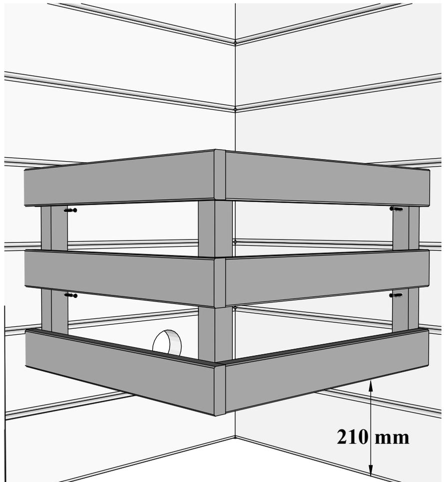
If possible, adjust the height of the heater protection
