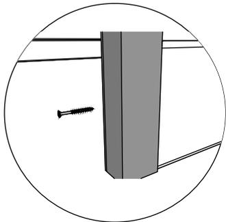
Drive the screw in pre-drilled
