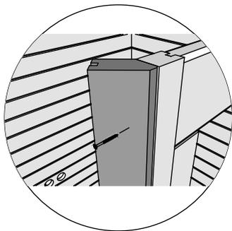
Drive the screw in pre-drilled
