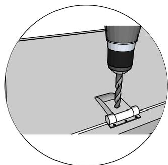
Drill the marked points for the hinges
