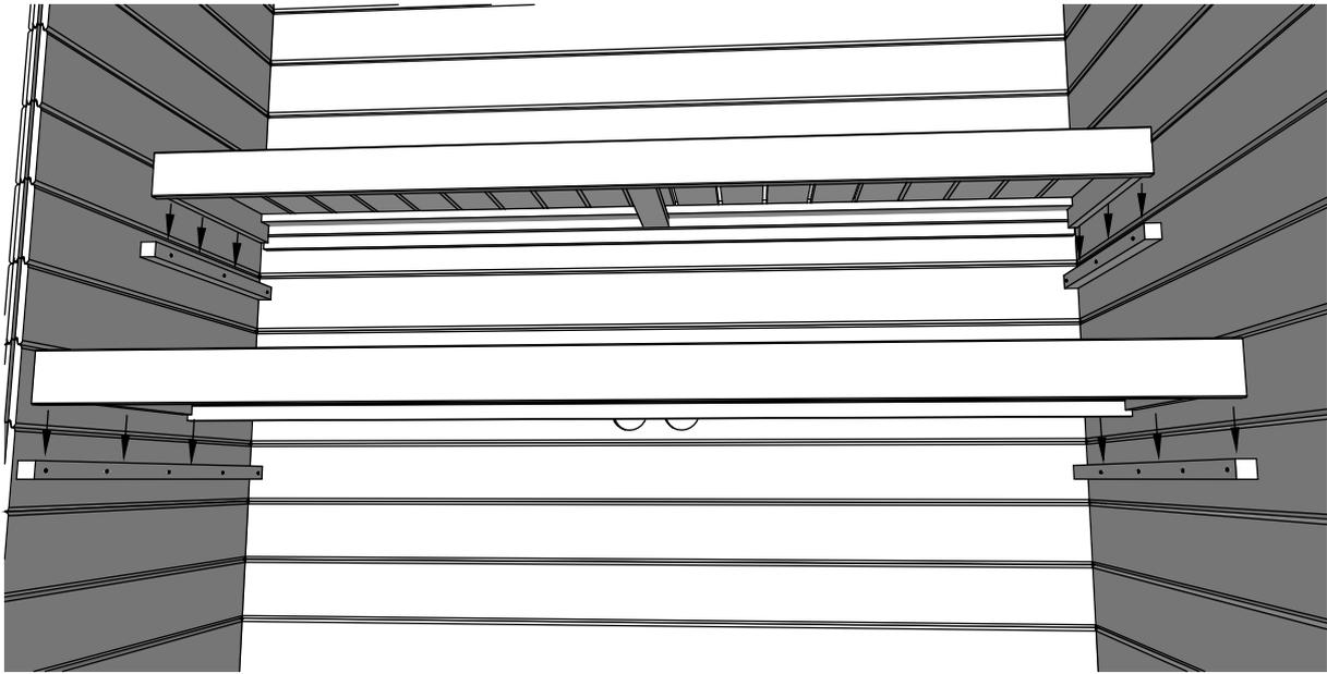
**Place the upper sauna bed on the holder and fasten with screws.
