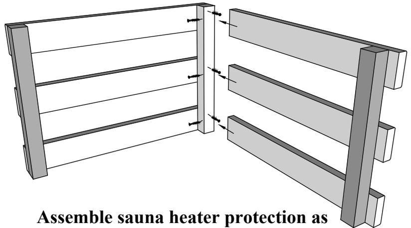
Assemble sauna heater protection as
